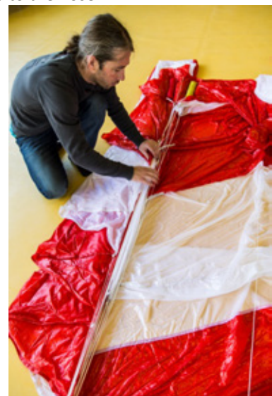
Pic. 78-79 Slide excess material back into the folded panels
