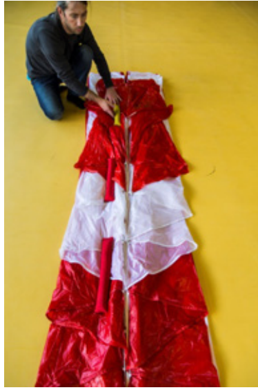
Pic. 92 Weighting down one wing half
