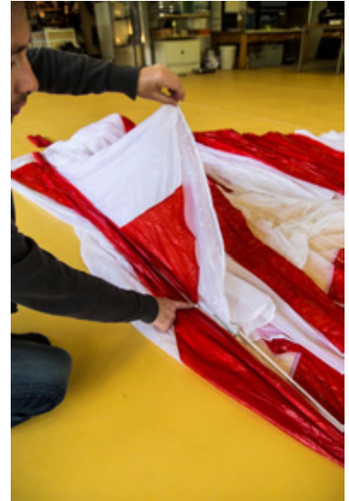
Pic. 64 Put the line attachment point on the middle lines and hold it there
