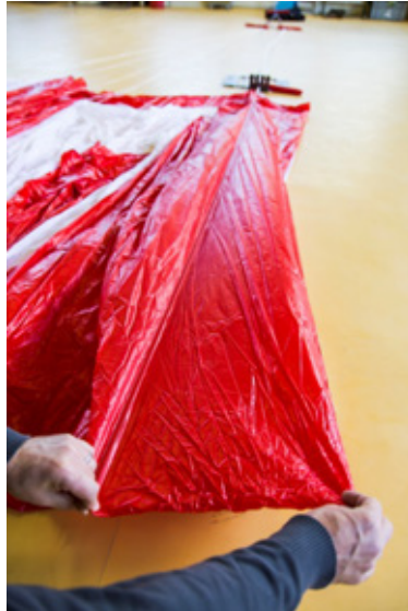
Pic. 72 Lay panel #4 to the outside and halve it (one fold)
