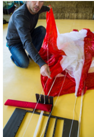
Pic. 55 Put this line in the line separator (weight)
