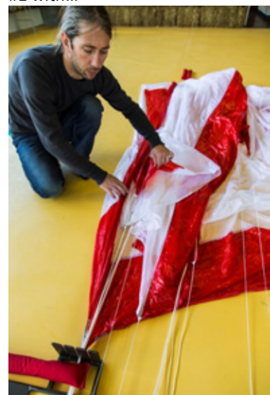
Pic. 61 Line #1 on the centreline!
