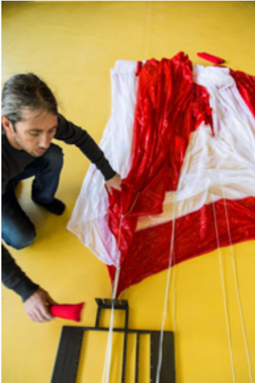
Pic. 71 Line #4 in the line separator
