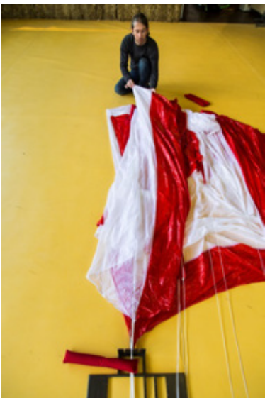
Pic. 68 Line for panel #3 in the line separator
