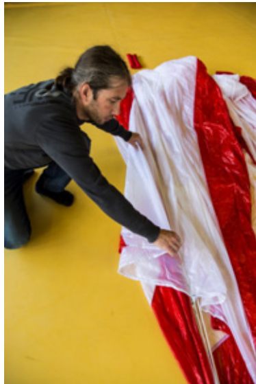
Pic. 66 Fold panel #2 in an S
