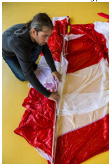
Pic. 78-79 Slide excess material back into the folded panels
