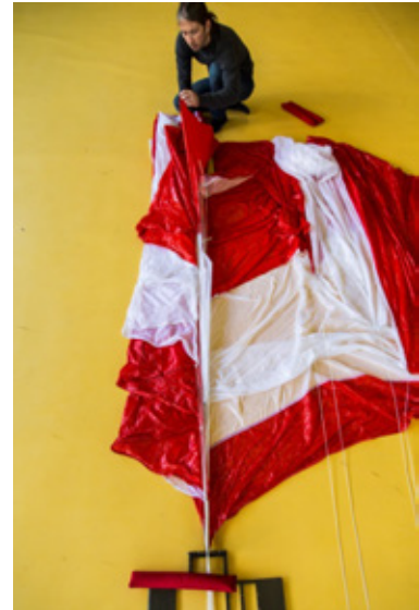
Pic. 75-77 Fold the remaining panels up to the nose...
