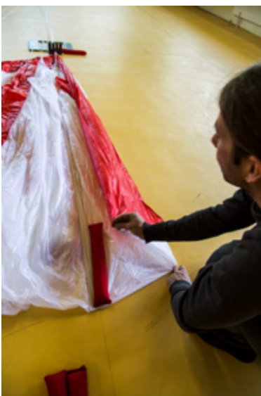
Pic. 59/60 ...with an S - 2 folds (for Beamer 3 small only halved)
