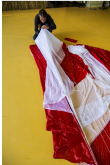
Pic. 75-77 Fold the remaining panels up to the nose...
