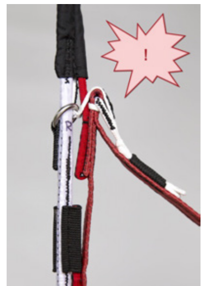
Pic. 16 Stow the brake stick outside the metal ring!
