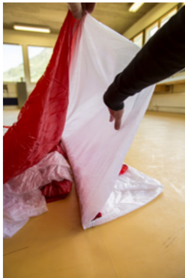
Pic. 69 Stretch panel #3 to the side; halve it with one fold.
