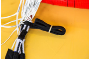
Pic. 134-137 Fold the interconnector in half twice and secure with an elastic band
