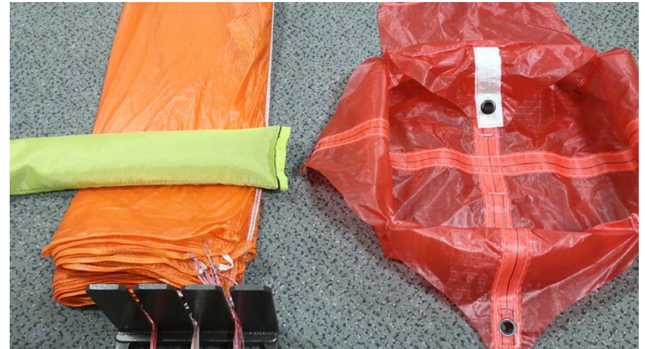
Now the canopy is folded to the correct width of the container.
