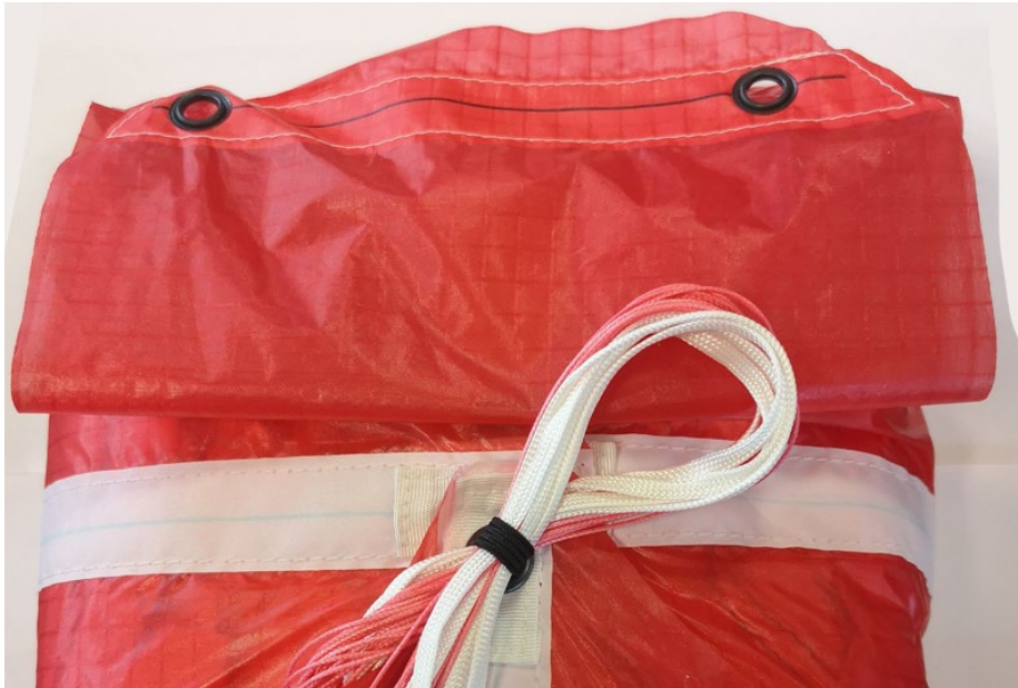
Close the deployment bag with a loop of suspension lines of 5 to 6 cm (approx. 3 fingers wide).
