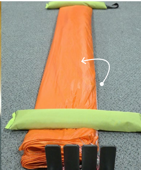
Double over the canopy a further time along the centre axis.
