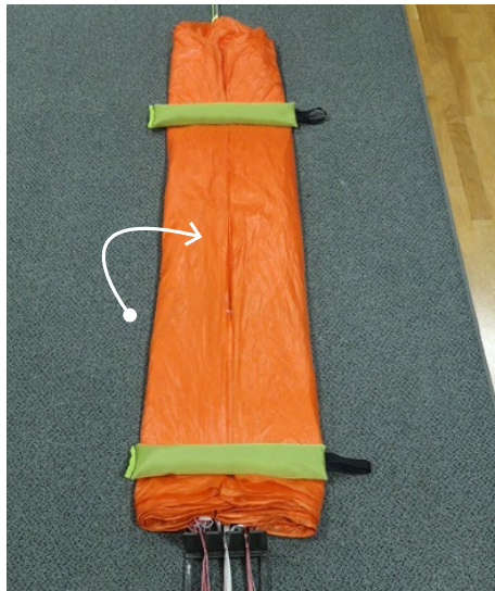
Double over the left canopy half towards the centre axis. Packing weights help with fixation.
