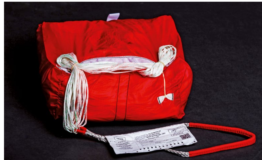
Close the deployment bag by securing the fourth leaf with the remaining lines.
