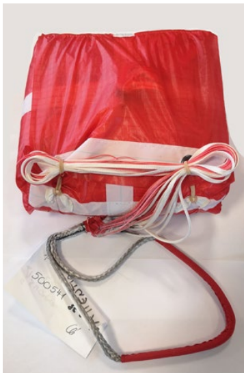
Close the deployment bag with a loop of suspension lines of 5 to 6 cm (approx. 3 fingers wide).
