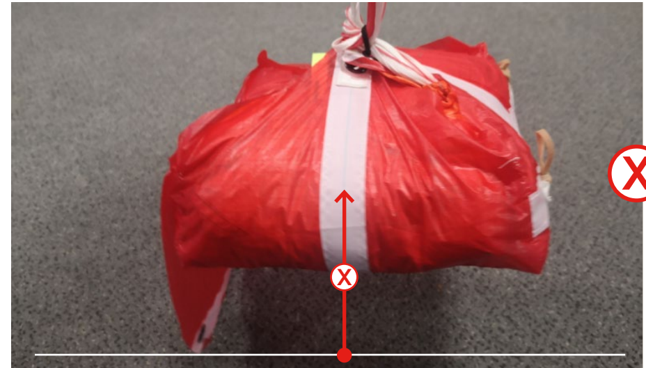
False: The parachute, packed in the deployment bag, can be lifted by the bridle.
