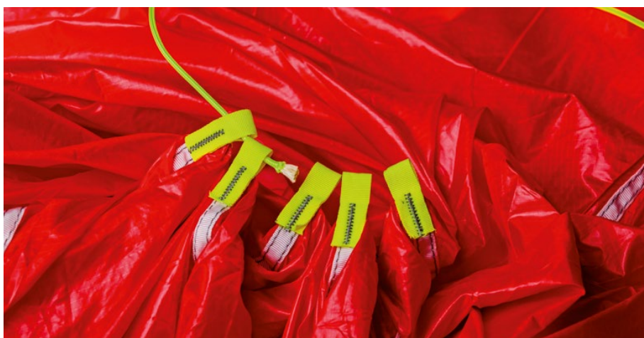
Release the packing loops and remove the piece of packing line.
