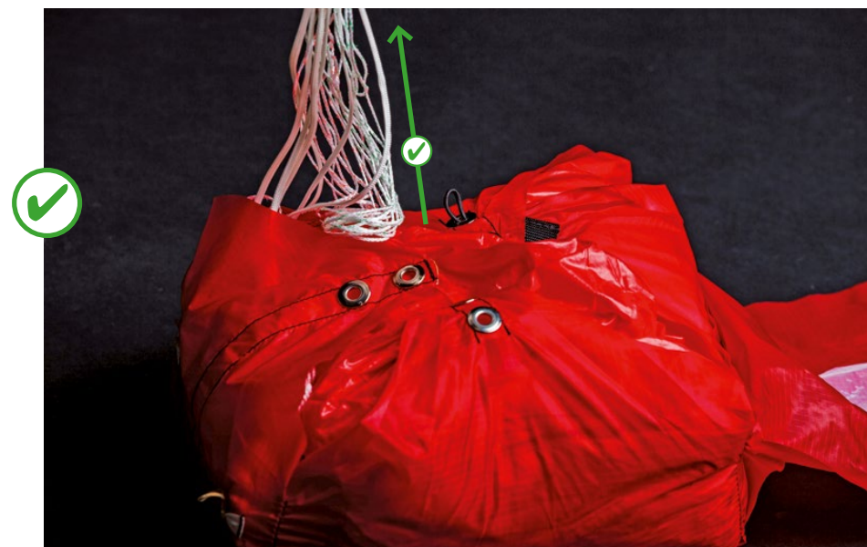
Correct: The parachute, packed in the deployment bag, cannot be lifted by the bridle.
